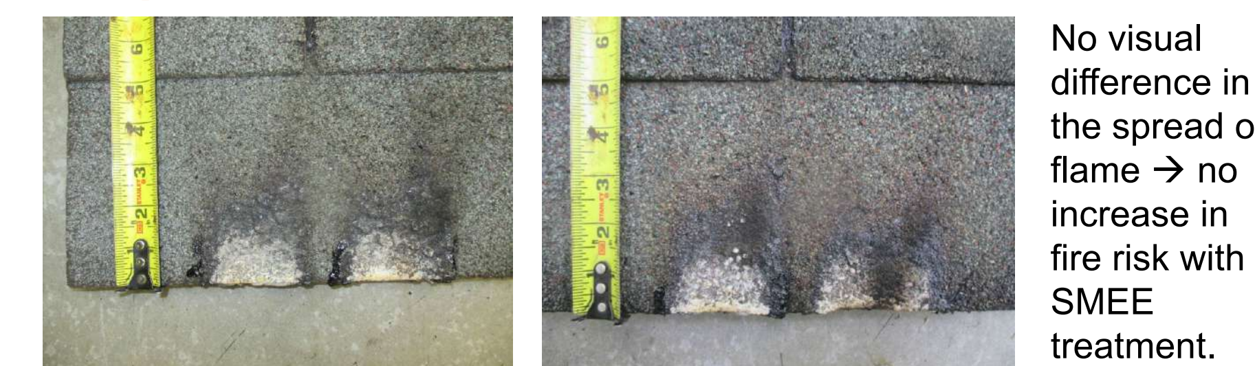
Fig. 7 Spread of flame in asphalt shingles decks.
