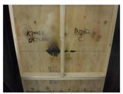
Phota No. 9 Test #2 Underdeck During Test
