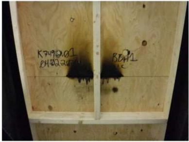
Phota No. 4 Test #1 Underdeck During Test
