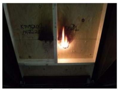
Photo No. 5 Test #1 Underdeck Ignition
